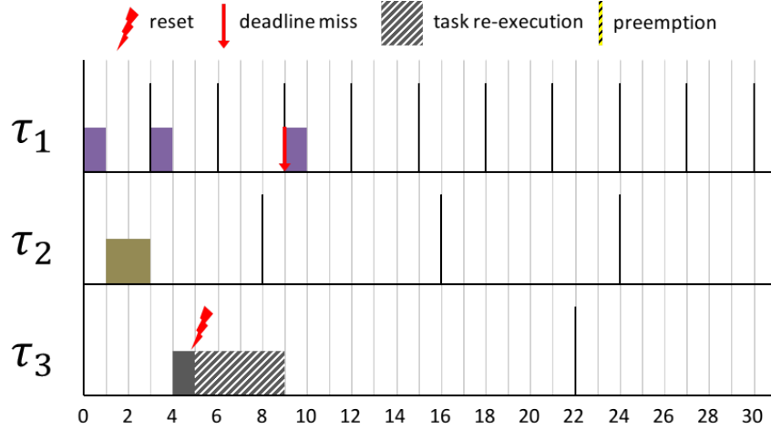
Fig. 2: Example of fully non-preemptive system with 3 tasks \tau_1 = (1, 3) ; \tau_2 = (2, 8) ; \tau_3 = (4, 22) , and restart at t = 5 - \epsilon ( C_r = 0 ). Restart and task re-execution causes a deadline miss at t = 9 .
