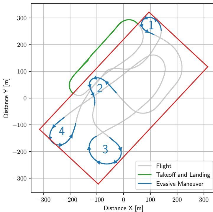
**Figure 20.** The real-life flight path of the Avistar UAV deployed with the uavAP autopilot with geo-fencing; red shows the geo-fence, blue shows the evasive maneuvers labeled from 1-4 (note that the boundary slack value is 5 meters and velocity is 20 m/s).
