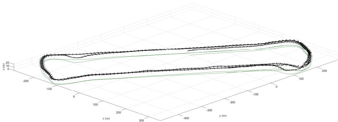
Figure 22. The trajectory of the UIUC-TUM Solar Flyer during a repeated level race track maneuver (note that the aircraft is plotted 6x scale every 0.5 sec).
