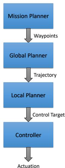
Figure 1. Planning and control stack implemented in uavAP.
