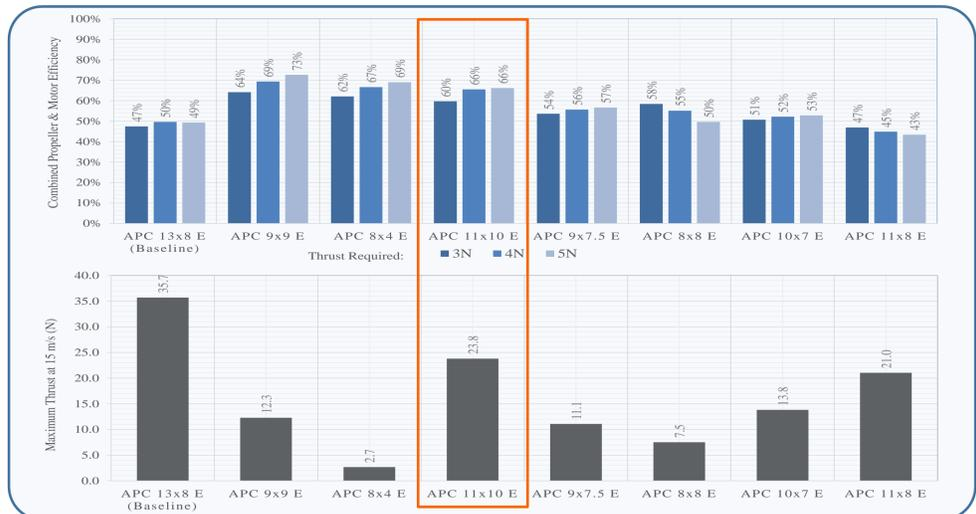
Simulations were then conducted for field coverage and long-distance, multi-site inspection missions with thousands of aircraft compatible motor-propeller combinations. The results showed power saving of 50-75% compared to the baseline combination.
